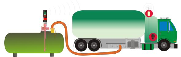
The system automatically monitors the treshold of the LPG tank. Upon reaching the maximum filling capacity the process is automatically stopped.
